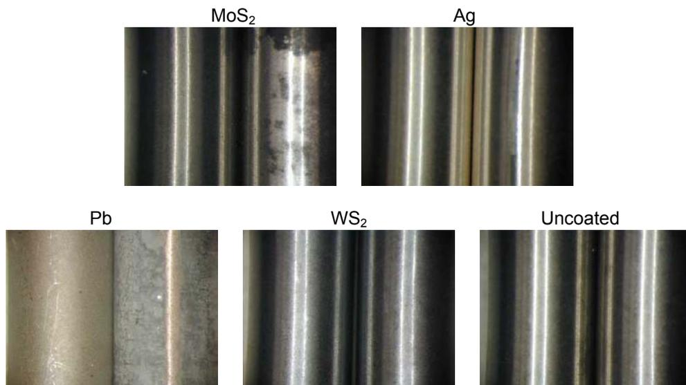
**Figure 2. Salt Fog Test Results**
