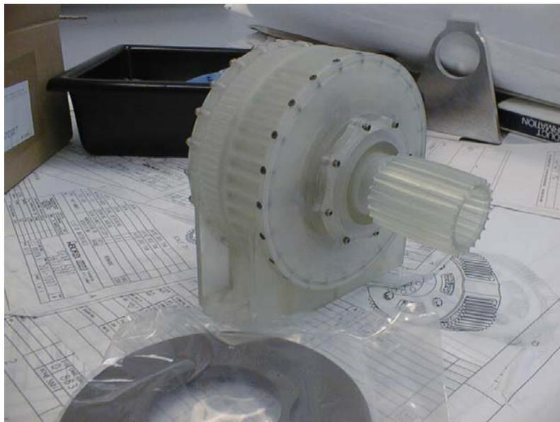
**Figure 3. SLA Model of LPA**
