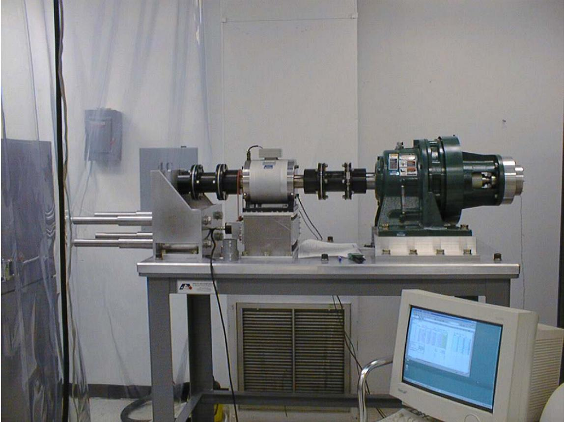
**Figure 7. Dynamometer Portion of Test Apparatus**
