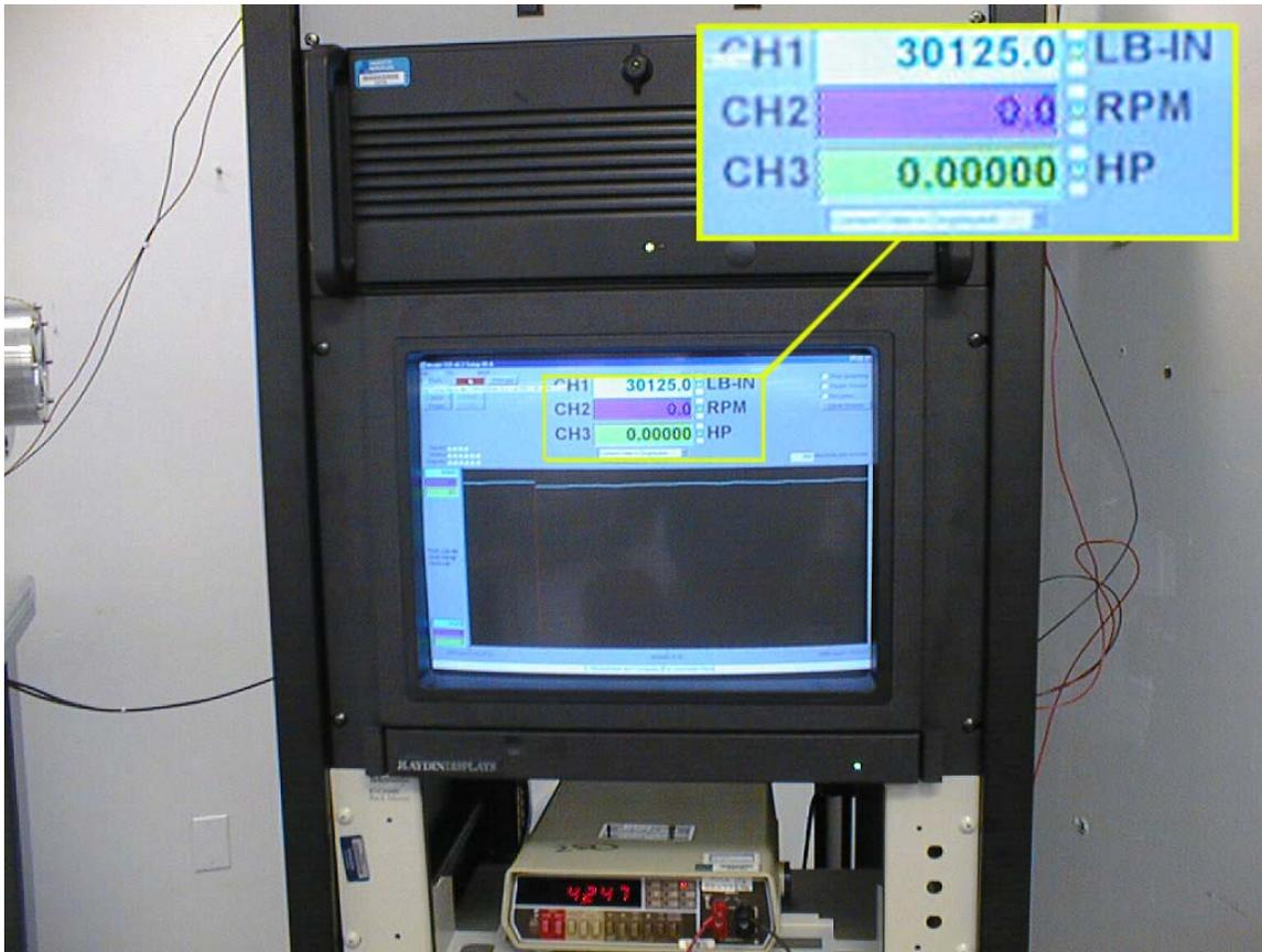
**Figure 4. Moment Of Truth, Actuator Output at 3390 N-m**
