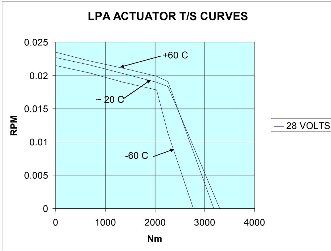
Figure 8. Actuator Torque/Speed Curve vs. Temperature
