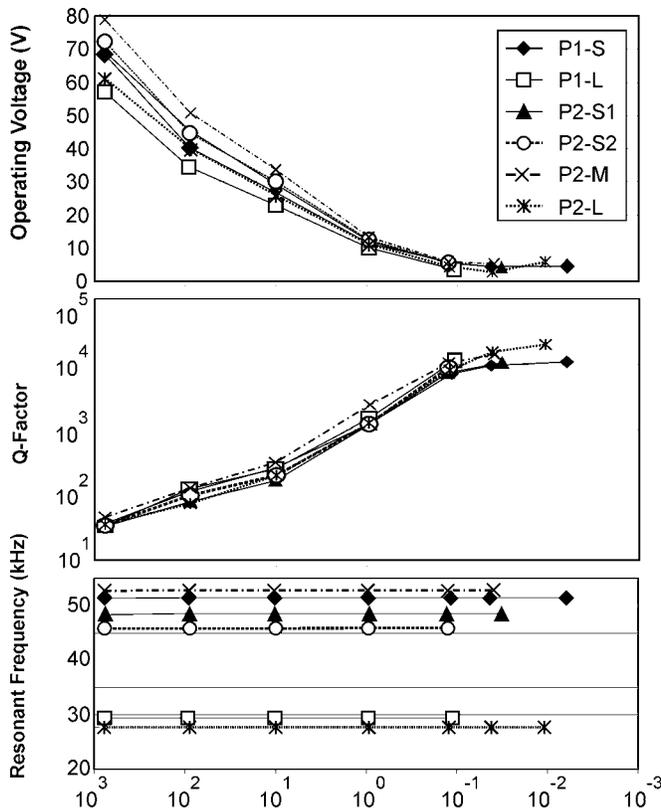
**Figure 4. Required operating voltage, device Q-factor, and resonant frequency plotted versus partial pressure of air in the microprobe station. All six oscillator geometries show the same basic response, with full vacuum-type motions not being experienced until the pressure is below ~13 Pa (0.1 Torr).**
