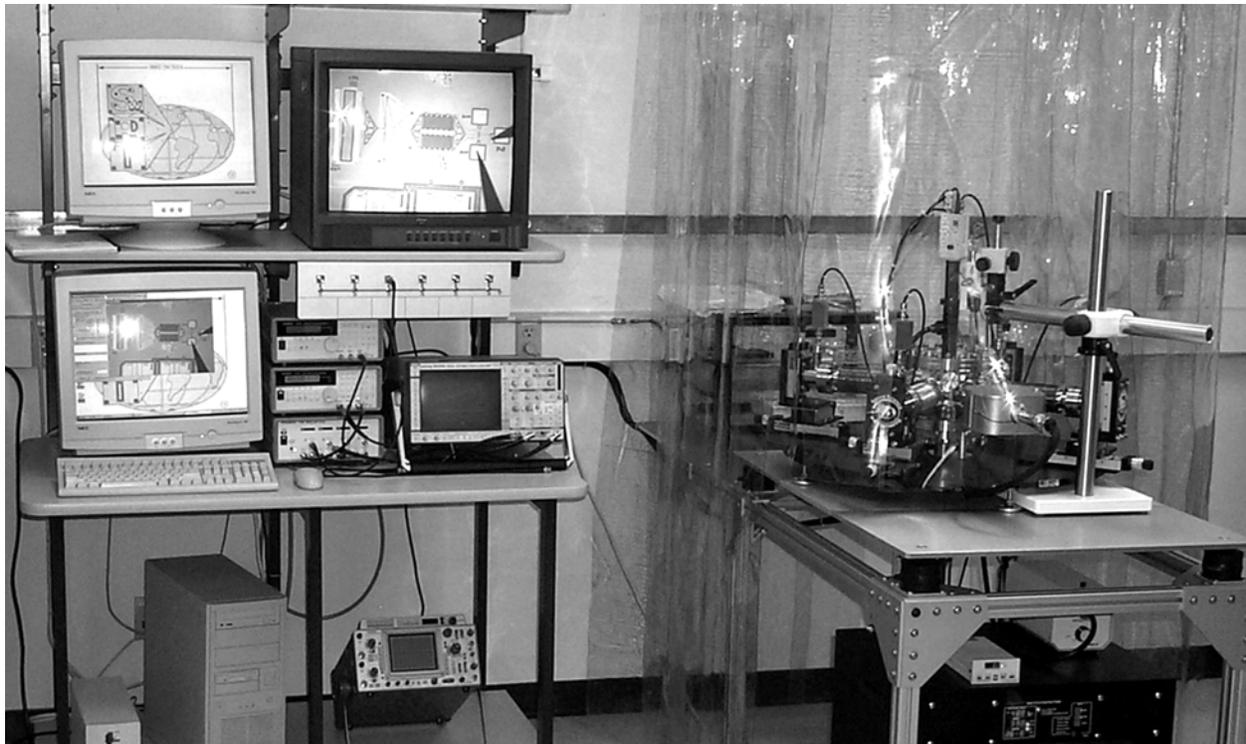
**Figure 1. The SwRI MEMS development and test facility. The vacuum microprobe station, mounted on pneumatic dampers, and nitrogen-purged storage cabinet are inside the down flow clean tent while the control computer, ARBs, ARB signal amplifiers, and high resolution direct-feed monitor are on the adjacent workbench.**
