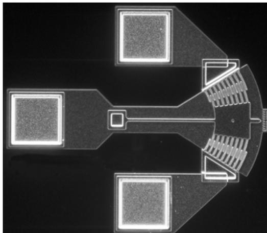
**Figure 3. Photograph of a medium-sized type oscillator device.**
