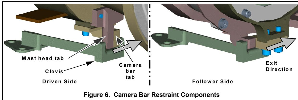
Figure 6. Camera Bar Restraint Components
