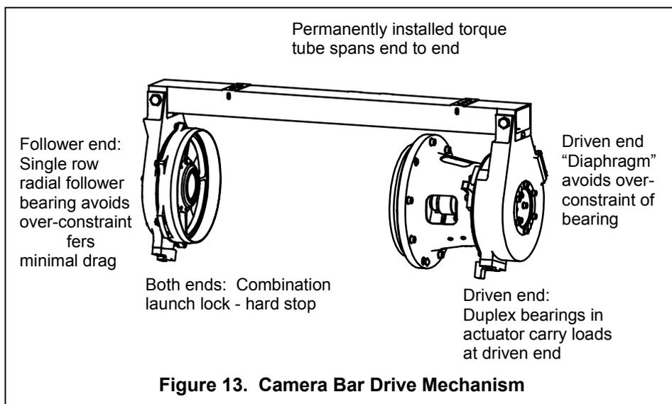
**Figure 13. Camera Bar Drive Mechanism**
