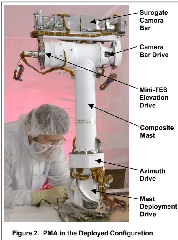
**Figure 2. PMA in the Deployed Configuration**
