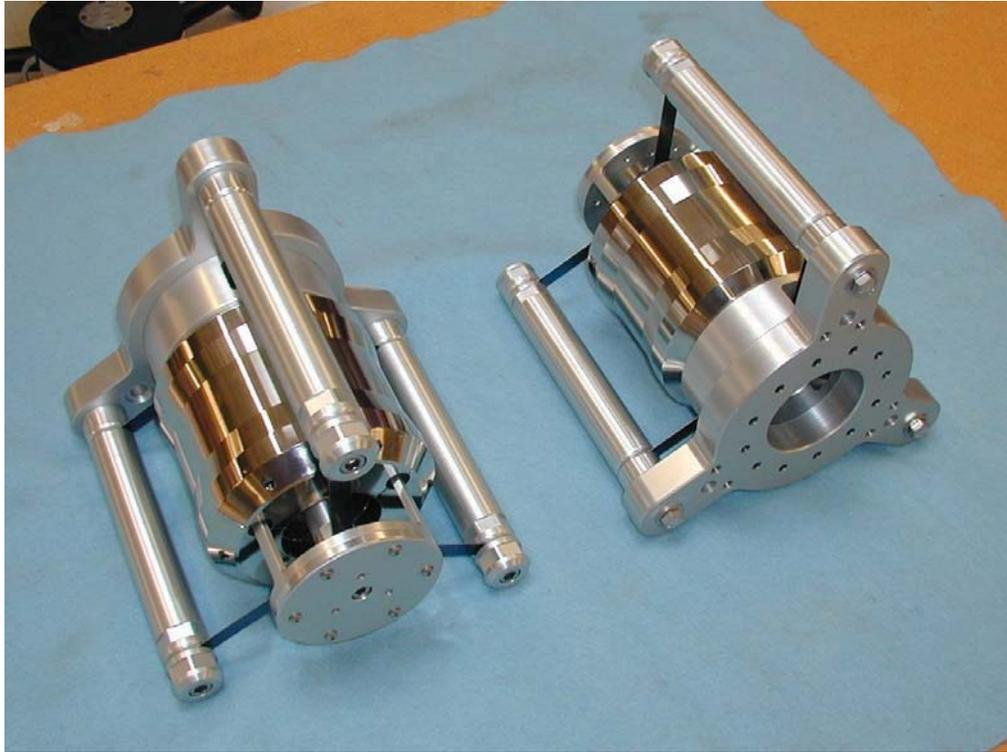
**Figure 9** Passive magnetic dampers for payload pendulum modes
