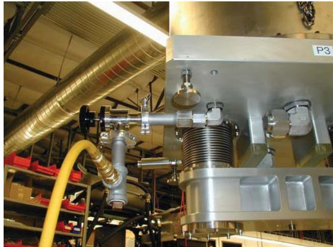
**Figure 14 Low-leakage vacuum valve used in leak rate tests**
