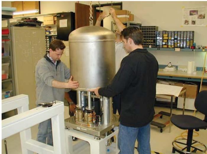
**Figure 6 Trial-fitting of vacuum housing onto suspension device.**
