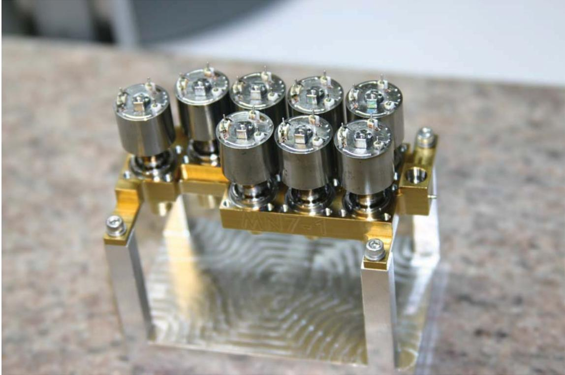
**Figure 7 - Flight Microvalves Welded into a Flight Manifold**
