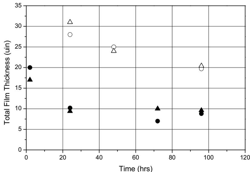
**Figure 4. Total Film thickness (in microinches) as a function of cumulative time operating at 6000 rpm with neat base oils formulated with TCP. Open symbols represent Coray and filled symbols represent Pennzane. Triangles are the results from the load cell and circles are the results from the displacement sensors.**
