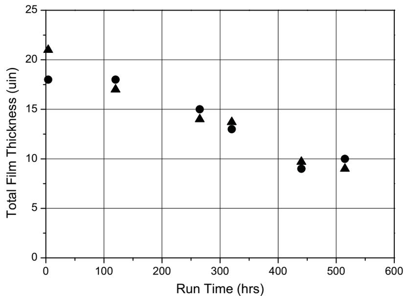
**Figure 6. Total Film thickness (in microinches) as a function of cumulative time operating at 6000 rpm with a grease pack of 0.14 g Rheolube. Triangles are the results from the load cell and circles are the results from the displacement sensors.**
