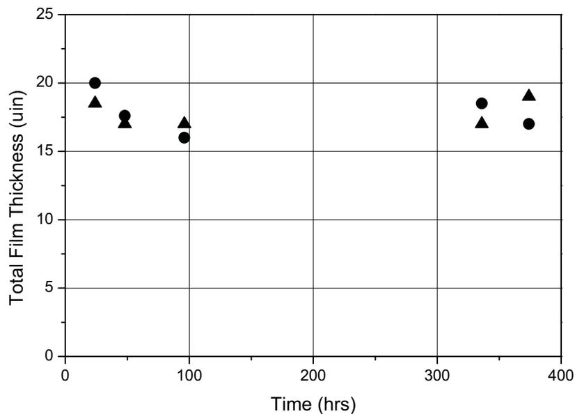
**Figure 5. Total Film thickness (in microinches) as a function of cumulative time operating at 6000 rpm with a grease pack of 1.1 g Rheolube. Triangles are the results from the load cell and circles are the results from the displacement sensors.**
