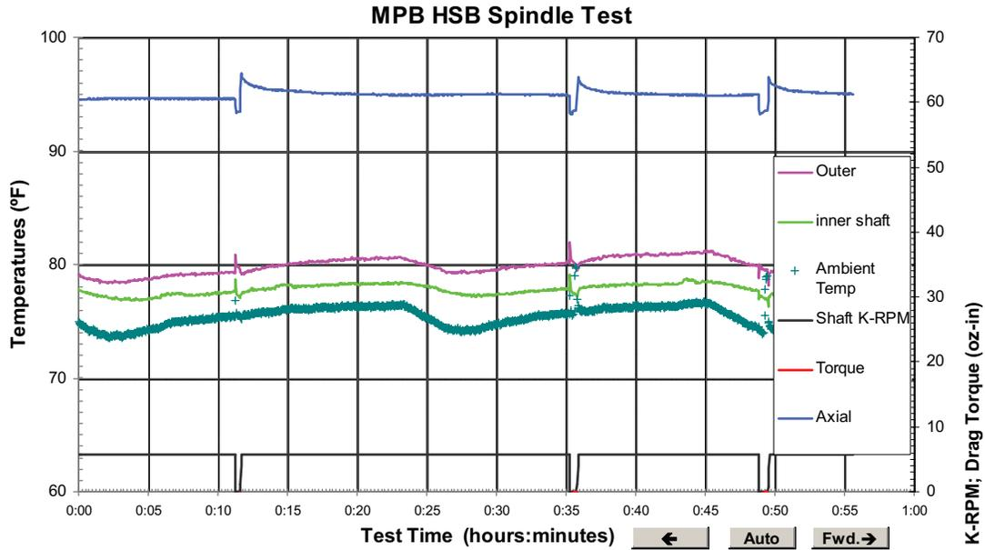
**Figure 3. An example of raw data. The top data stream shows the axial load that is used to determine bearing deflections. The three data streams bundled near the center are, from top to bottom, temperatures of the outer ring, inner ring, and laboratory ambient.**
