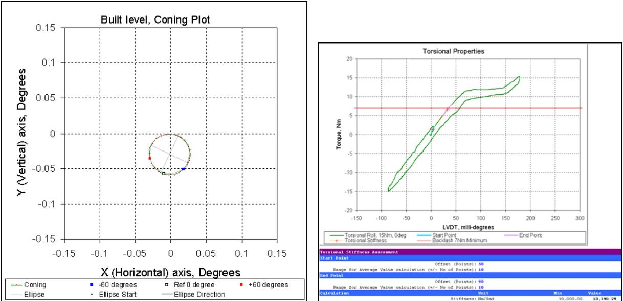
Figure 7: Left = Coning measurement, Right = Stiffness + Backlash measurements
