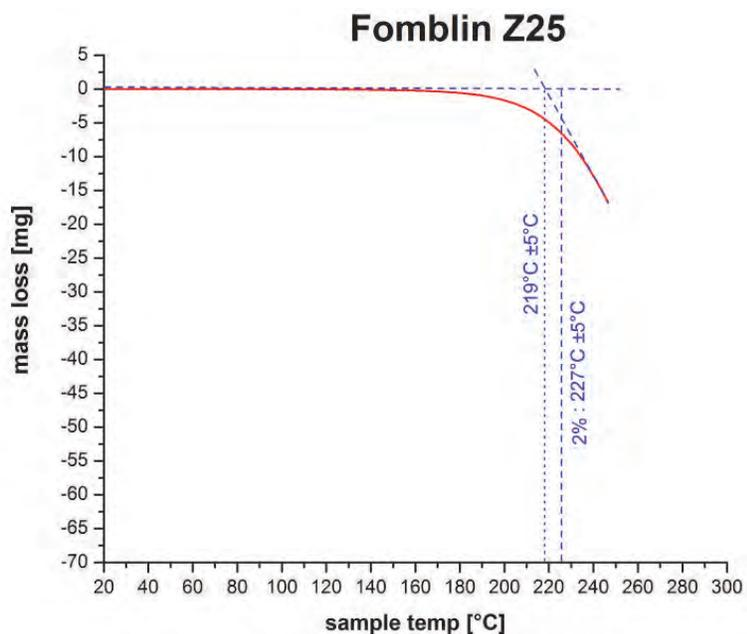
**Figure 5. Z25 sublimation test under high vacuum.**
