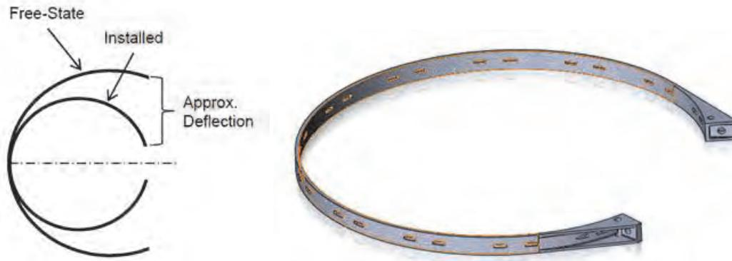
**Figure 4: One-Piece Aluminum Band Machining**
