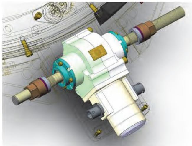
**Figure 3: 13,500-lb (60-kN) Clamp-Band Opening Device (CBOD)**
