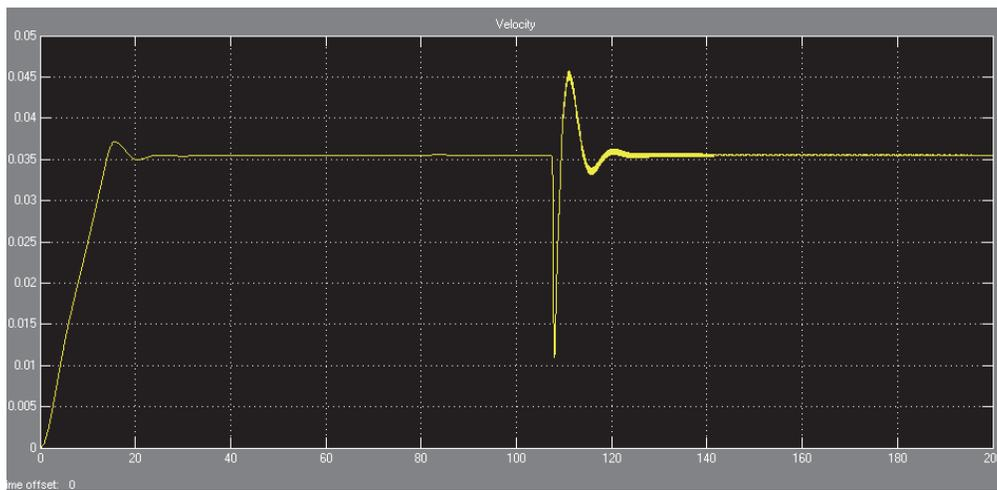
**Figure 19. Velocity versus time plot with no deadband**
