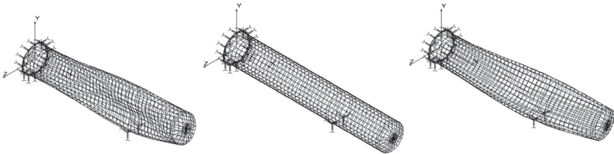
**Figure 6. First three modes in the stowed configuration**
