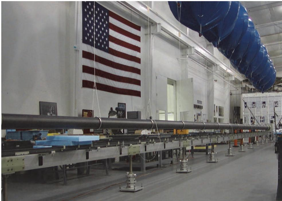
**Figure 7. Deployed stiffness test configuration**
