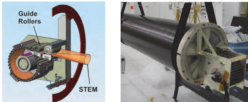
**Figure 3. STEM device used for TTM deployment/retraction**
