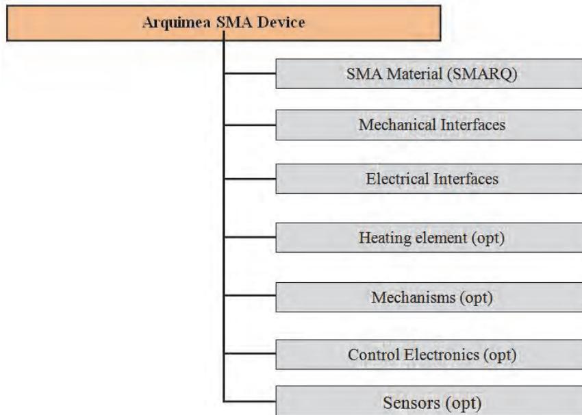
**Figure 2. Block diagram of Arquimea SMA Device.**
