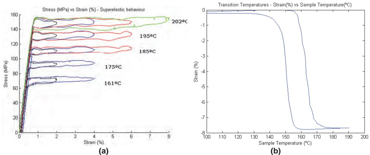
**Figure 5. Results of strength characterization and transition temperature test: (a) reconditioning force – superelastic behavior; (b) SMARQ Transition Temperatures - Strain vs. Temperature. Actuation above 125°C is shown.**
