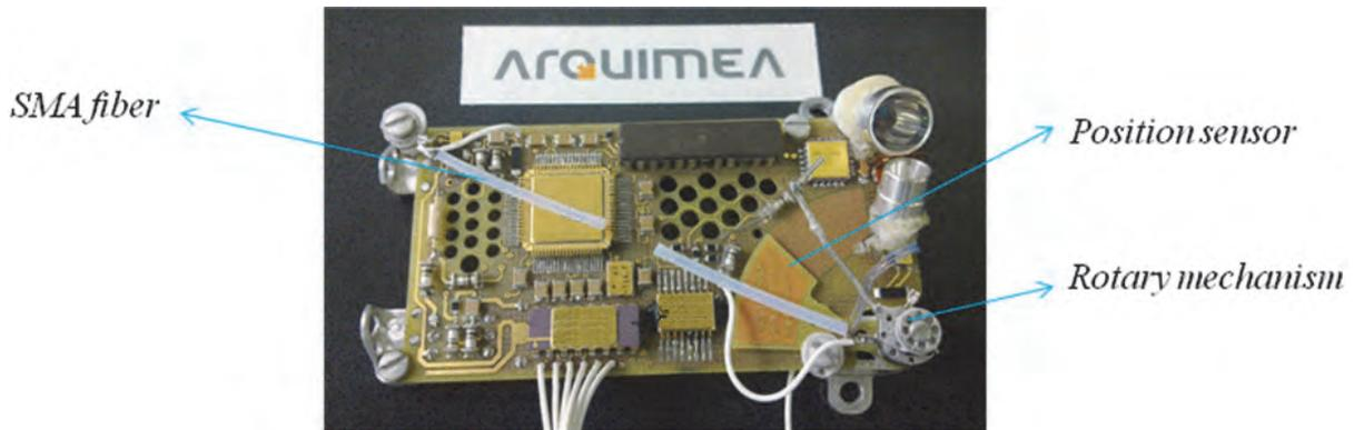
**Figure 3. Qualification Model of the Dust Sensor**
