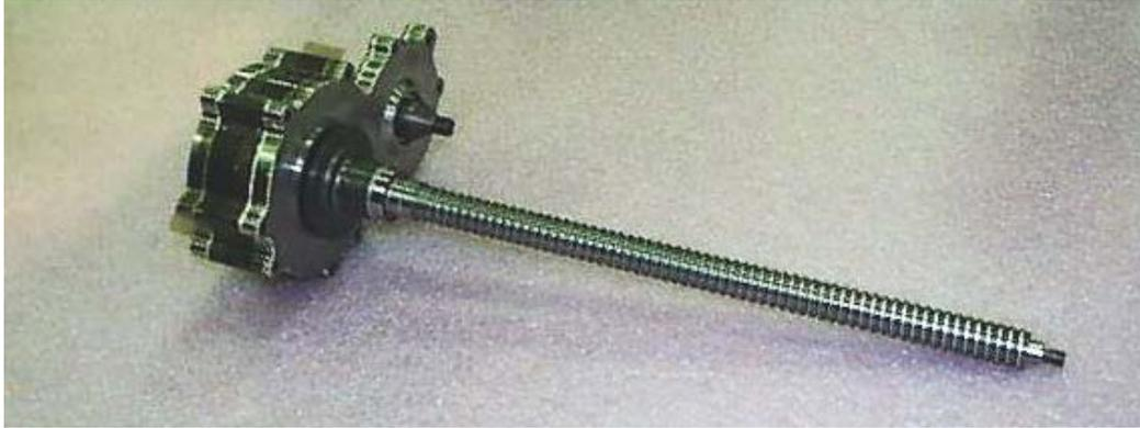
**Figure 4. SSRMS LEE Rigidized Gearbox With Ballscrew, Scale: ballscrew = 18-in long (46 cm)**
