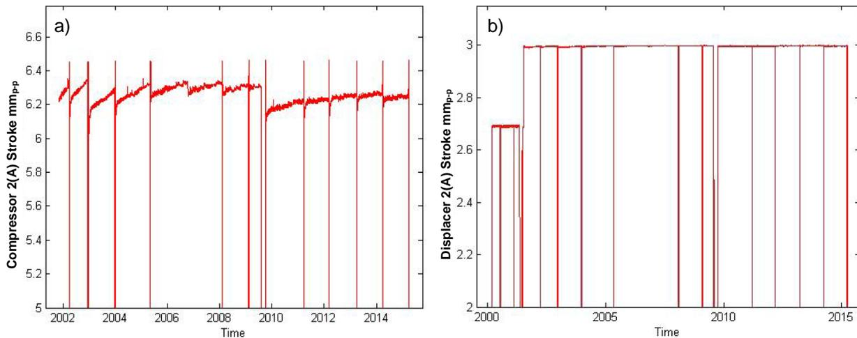
**Figure 10. Cryocooler Displacer and Compressor Displacement Over Lifetime**
