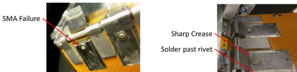
Figure 6. SMA Hinge Spring Failed Flight Attachment
