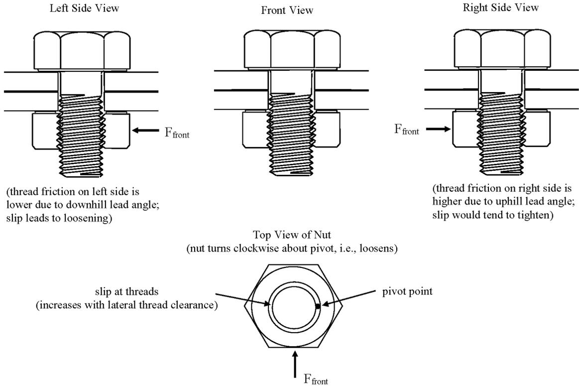
Figure 1. Bolted joint with force applied to nut from front.
