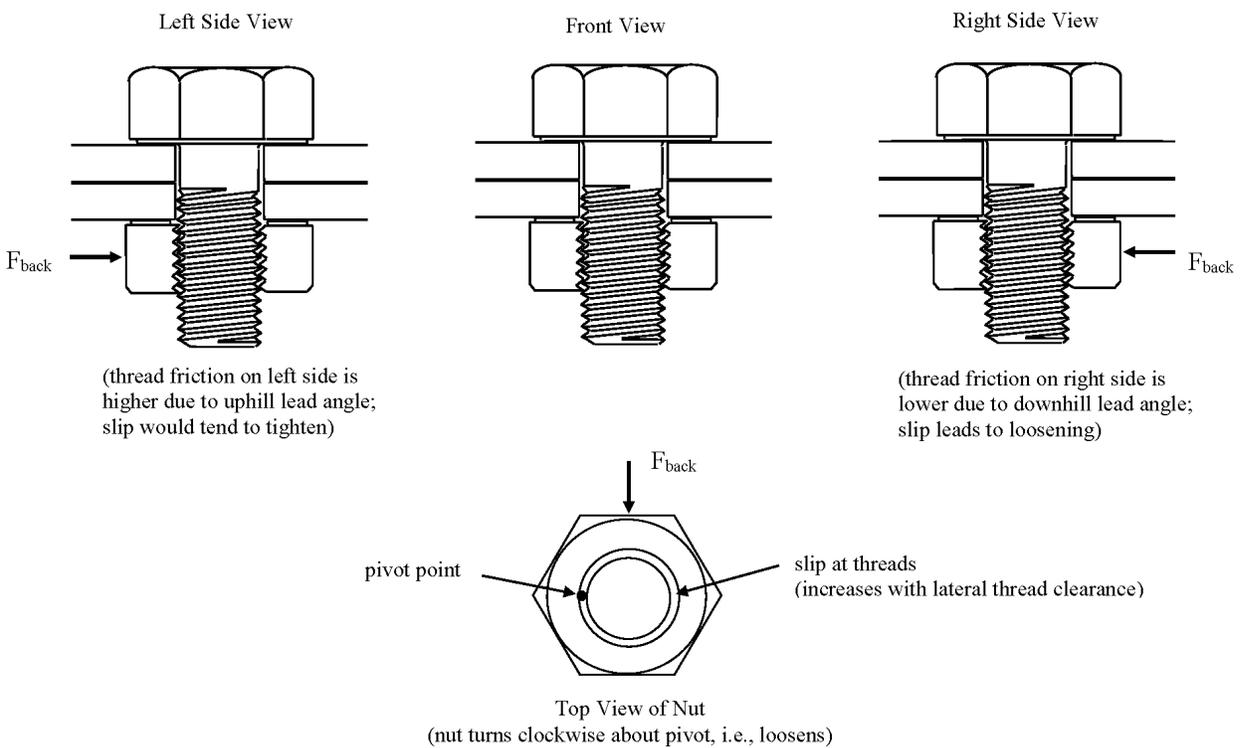
Figure 2. Bolted joint with force applied to nut from back.
