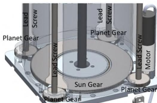
*Figure 6. Motorized Deployment System Components*
