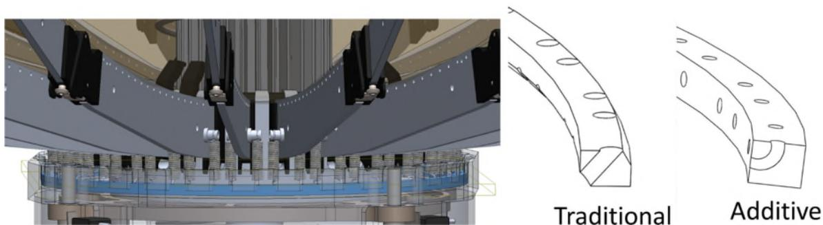
*Figure 4. An Additively Manufactured Spring Ring Allows for Unique Features*
