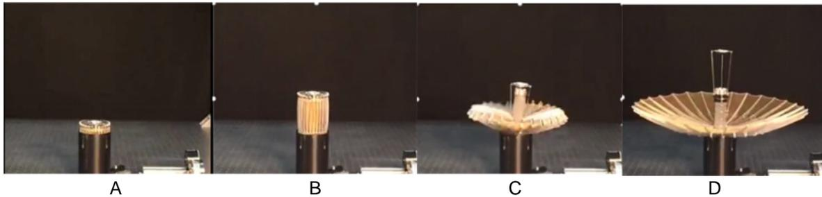
Figure 5. Antenna Deployment Via Gas Power
