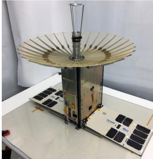
Figure 8. Flight KaPDA Installed with the Tyvak Spacecraft
