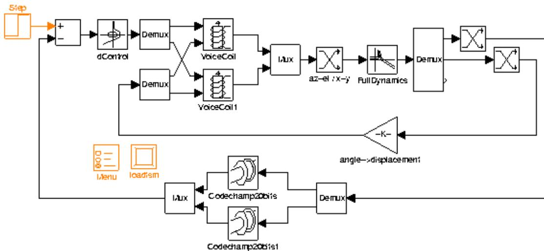
Figure 13 - FSM acquisition control loop model.
