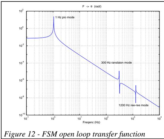
Figure 12 - FSM open loop transfer function
