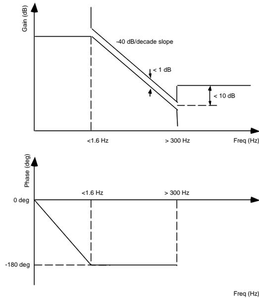
Figure 5 – FSM required frequency response
