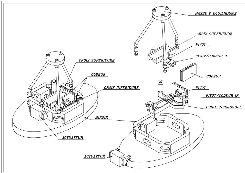
Figure 8 - FSM architecture
