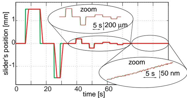
Figure 2: Illustration of the remarkable dynamic properties of these actuators (from nanometers to millimeters). Actually, the accuracy of the system is limited to 5 nm by the resolution of the position sensor (interferometer).
