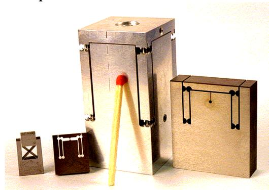
Figure 6: Examples of monolithic flexures. From left to right : cross spring pivot (tempered steel); linear stage with 4 necked down flexures  $25\mu\text{m}$  in thickness and a motion range of  $0.5\text{mm}$  (tempered steel), X Y  $\Theta$ Z stage (Perunal Aluminum alloy), linear stage. The match is  $50\text{mm}$  long.
