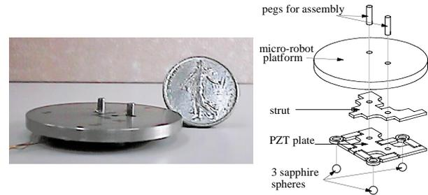
Figure 4: A 3 degrees-of-freedom mobile micro-robot.
