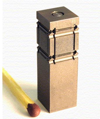
Figure 7: Compact monolithic XY stage with integrated flexible bellow (tempered steel). The flexible parts are  $25\mu\text{m}$  in thickness, the motion range is  $0.5\text{mm}$ . The part is  $30\text{mm}$  in height.
