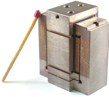
Figure 8: Compact monolithic serial XY stage. Motion range :  $\pm 1\text{mm}$ ; thickness of flexible parts:  $60\mu\text{m}$ ; material: titanium alloy TiAl6V4. The match is 50mm long.
