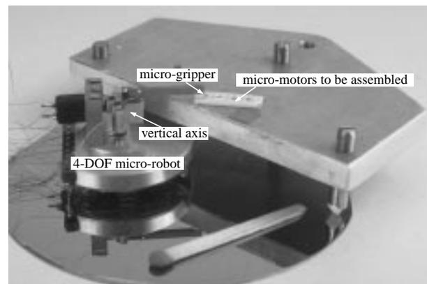
Figure 5: Micro-assembly system.
