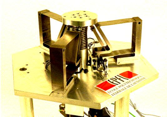
Figure 9: Orion X-Y-Z robot. This parallel robot is composed of three monolithic arms (tempered steel) connected to the moving platform on top. Each arm is actuated by a screw-nut system and a DC motor with encoder. The resolution of each axis is better than  $0.8\mu\text{m}$ . The linear motion range of the robot is  $\pm 5\text{mm}$ , the angular motion range is  $\pm 7^\circ$ . (The EPFL sticker is 60mm long).
