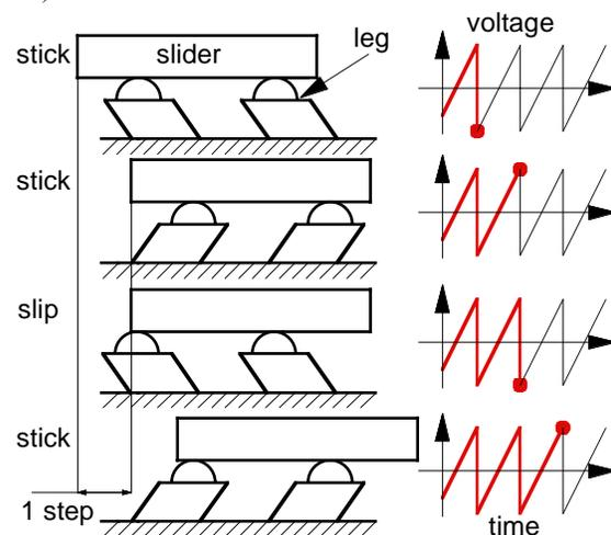
Figure 1: Stick and Slip Actuator, operation principle
