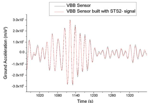
**Figure 6 : Quake occurred in Afghanistan, recorded by an STS-2 and by the VBB mock-up, on May 30, 1998. The signal was recorded in a seismic vault, in Saint-Maur, France. The quake has a magnitude of 6.9. The STS-2 outputs were used to compute the oblique output compared to the mock-up signal. Note however that the breadboard was operating without**
