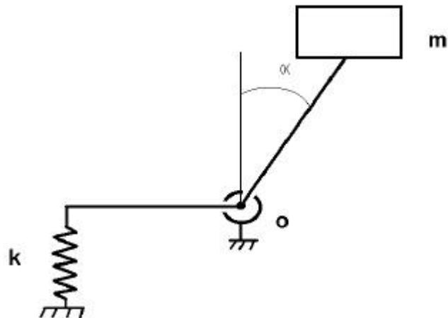
**Figure 2 : Principe of our 'inverted tilted pendulum'.**
