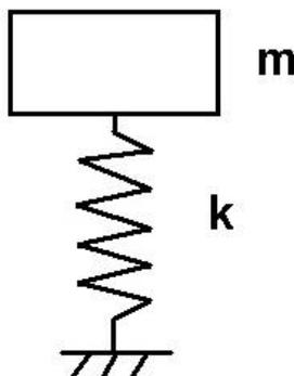
**Figure 1 : Principe of a vertical seismometer.**
