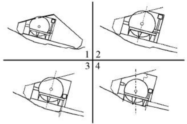
**Figure 8 :** Installation scenario of the seismometer. Objective is to uncouple the instrument from the lander and to assume a correct coupling with the ground.
