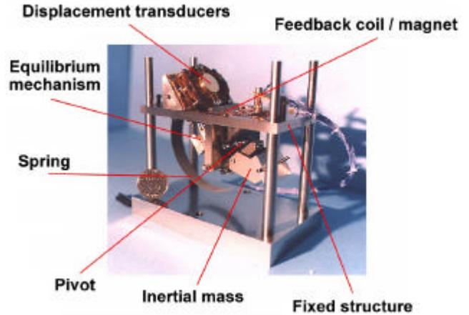
**Figure 5 : Mock-up of one axis sensor realized in 1997.**
