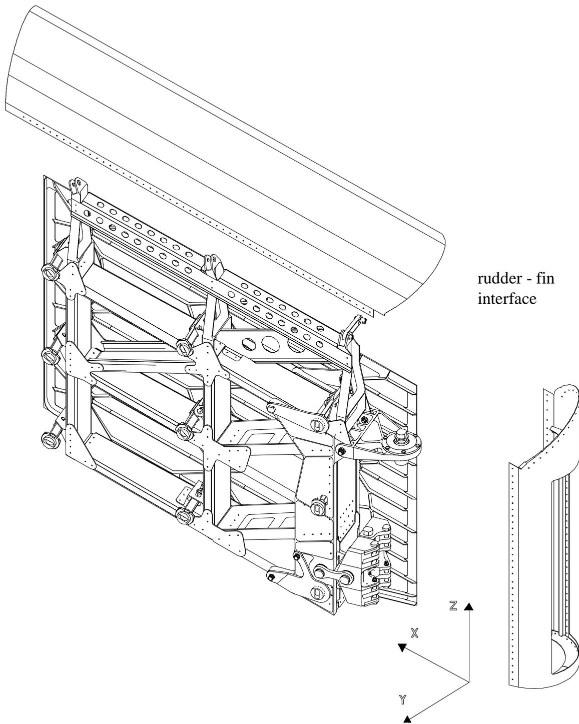
Fig. 3 Rudder frame, exploded view
