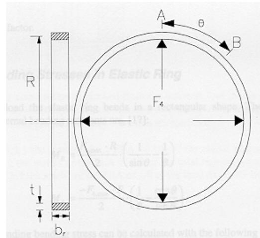
Figure 2 Outer Ring pre-stressed with 4 planets.
