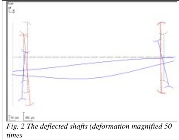
Fig. 2 The deflected shafts (deformation magnified 50 times)
