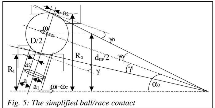
Fig. 5: The simplified ball/race contact
