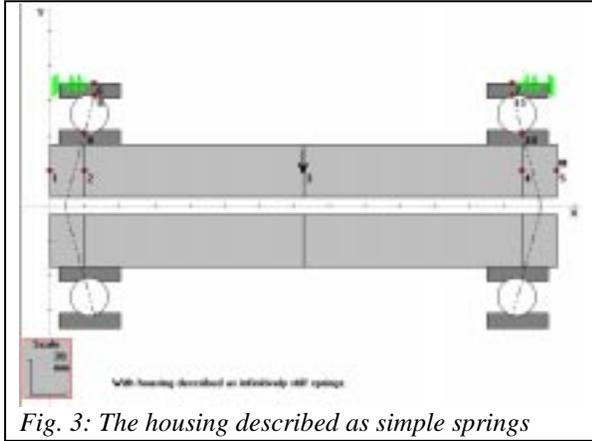
Fig. 3: The housing described as simple springs
