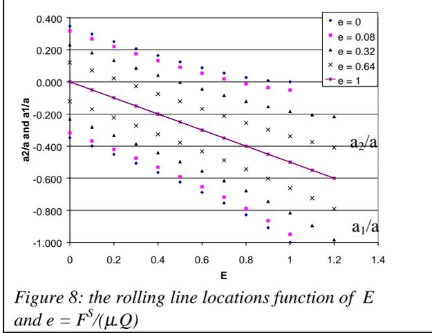
For  $E$  and  $e$  nil, the two rolling line are symmetrical and equal to  $\pm 0.347$ . For  $E$  larger than 1 and  $e$  small, only one rolling line is found,  $a_2/a = 0$ , the other one ( $a_1/a$ ) being out of the contact ellipse.
