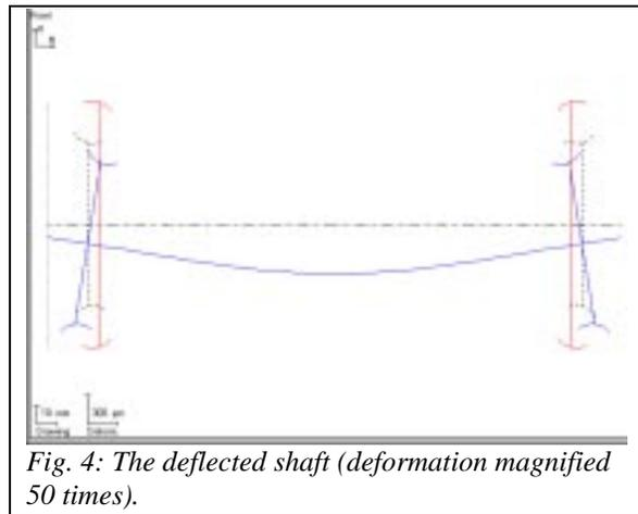
Fig. 4: The deflected shaft (deformation magnified 50 times).
