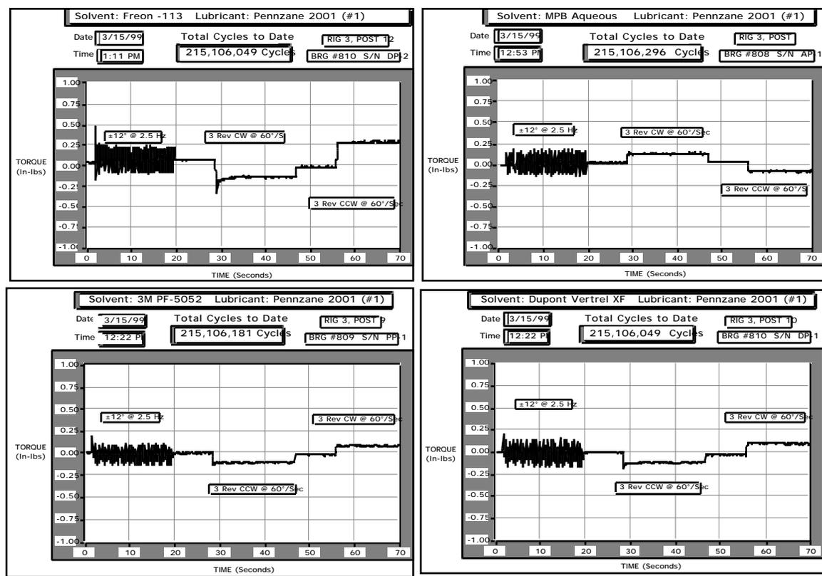
Figure 3 Four Solvents at 215M Cycles with Pennzane 2001
