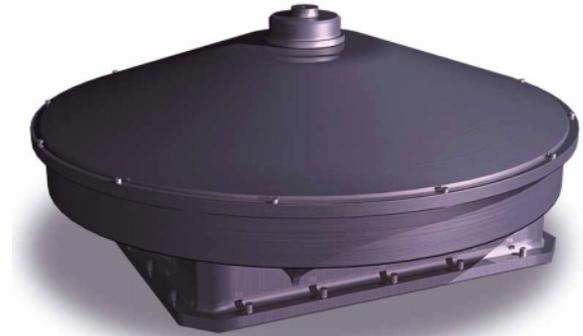
Figure 1 HR14 Reaction Wheel Assembly
