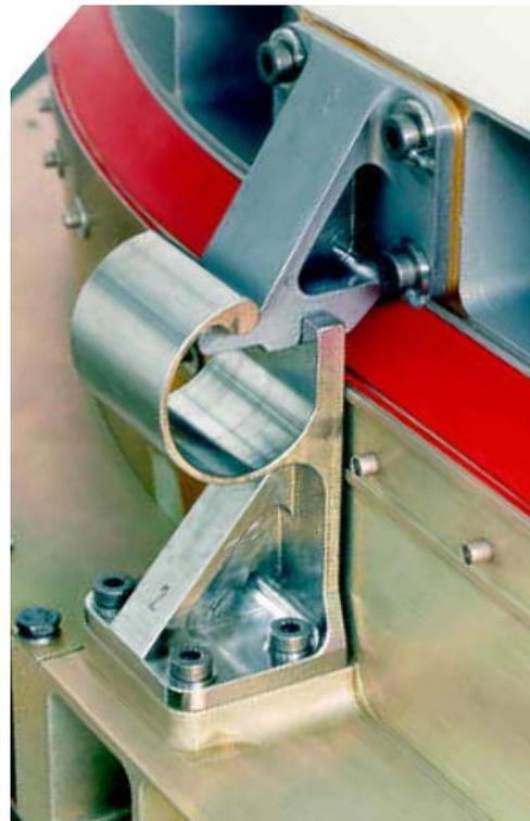
Figure 7. Flexible hinge mechanism, lateral view.
