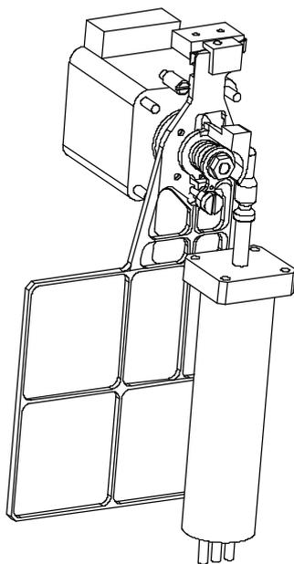
Fig. 3: VIRTIS-M Emergency Device (Actuated)
