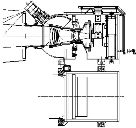
Fig. 8: NavCam Optical Head, cross section
