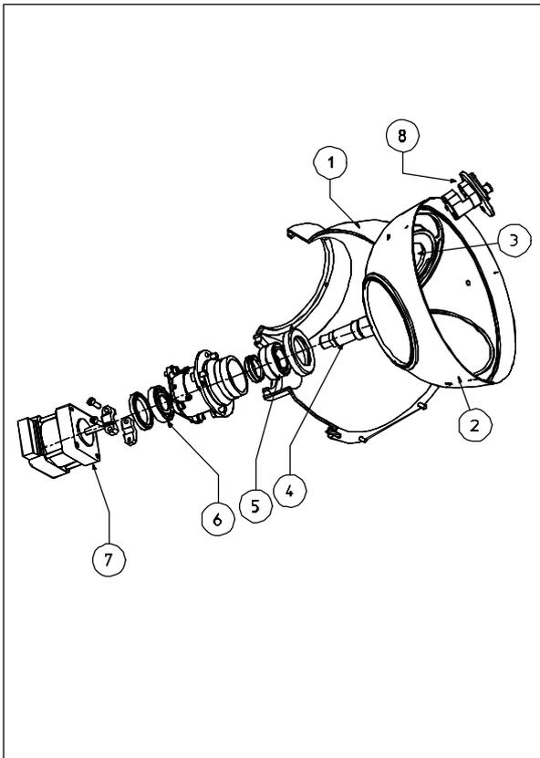
Fig. 10: NavCam Cover Mechanism, exploded view
