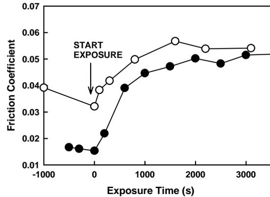
6 shows the friction coefficient of the RF and of the RF-H samples at the beginning of AO beam exposure. The AO beam exposure was carried out in the fluence of  $3.0 \times 10^{14}$  AO/cm<sup>2</sup>s at 1 Hz operation. *Figure 6 Change in friction coefficient of the sputter-deposited MoS<sub>2</sub> samples due to the AO beam exposure. Solid and open circles represent the data of RF and RF-H samples. AO flux is  $3.0 \times 10^{14}$  AO/cm<sup>2</sup>/s.*
