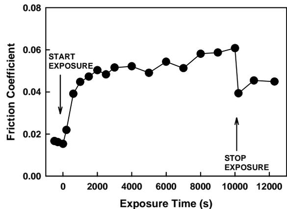
After starting the AO beam exposures, both samples indicated high friction coefficients of up to 0.06 at 3,000 AO. *Figure 7 Change in friction coefficient of the sputter-deposited MoS<sub>2</sub> samples due to the AO beam exposure. AO flux is 3.0 x 10<sup>14</sup> AO/cm<sup>2</sup>/s. A correlation between AO beam exposure and the friction coefficient is clearly obvious.*
