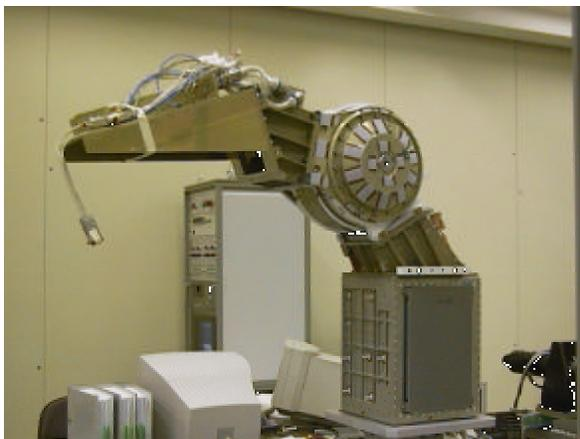
Figure 1: Elbow Assembly
