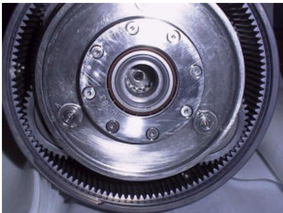
Figure 4: Planetary Gear of ERA Joint
