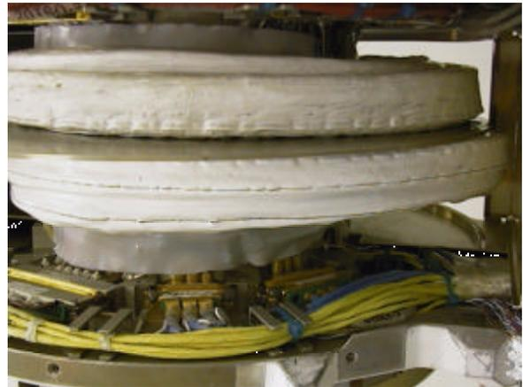
Figure 3: Ribbon Cables in Pitch-Type Joint
