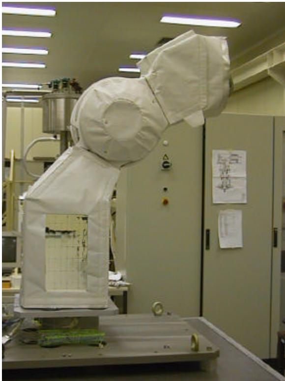
Figure 6: Elbow Assembly with MLI Blankets
