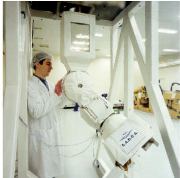
Figure 7: Wrist Assembly with MLI Thermal Blankets
