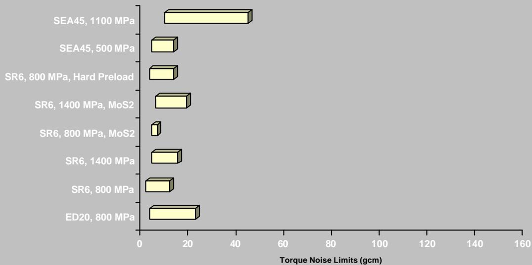
**Fig.3 Summary of 0-to-Peak Torque Limits for ED20, SR3, SR6 and SEA45 Ball Bearings Operating in Vacuum at 20 deg C**
