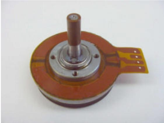
**Fig. 16** Piezo electric motor.
