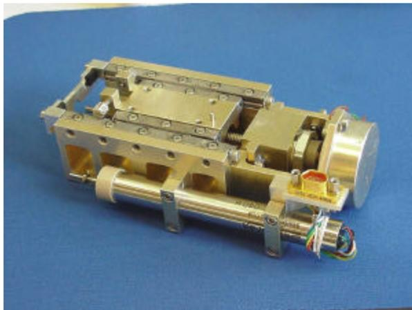
**Fig. 11** The translation stage with LVDT
