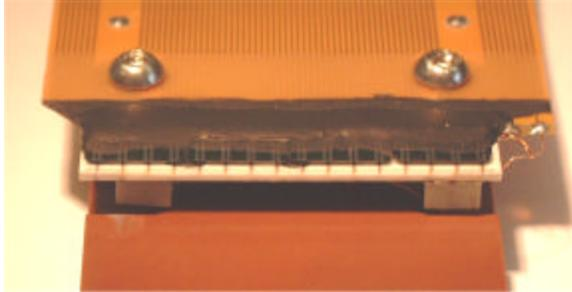
**Figure 4** The array with 16 cantilevers
