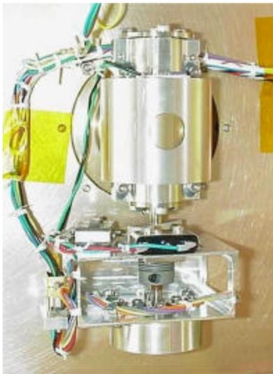
**Fig. 5** The shutter of the dust-intake system
