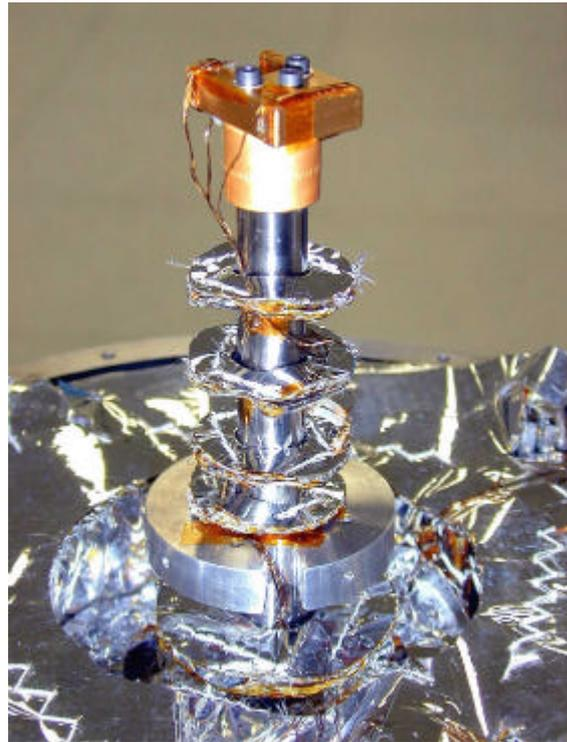
Figure 3. 10 K Cooler Cold-Tip with Temperature Monitor
