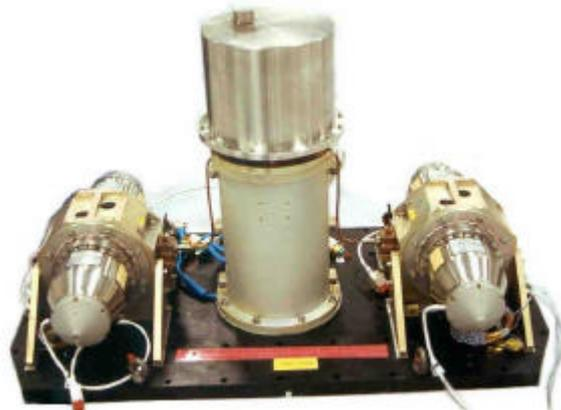
Figure 1. 10 K Closed Cycle Stirling Cooler System
