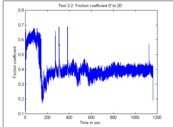
Figure 1.1: Friction trace with two main values for the friction coefficient
