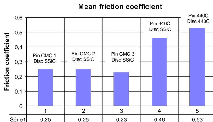
Figure 2: Comparison of friction coefficients
