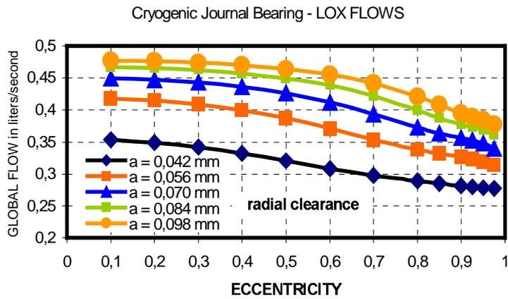
Figure 6: Influence of the radial clearance on recess flows
