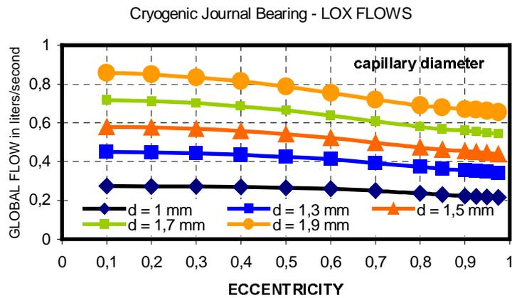
Figure 8: Influence of the capillary diameter on recess flows
