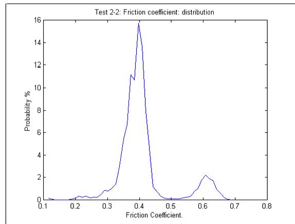
Figure 1.2: Statistical distribution of the friction trace
