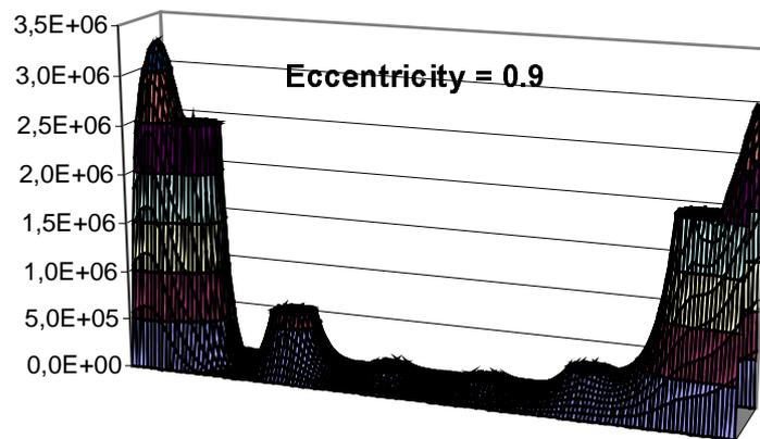
Figure 4: Pressure field in the sleeve
