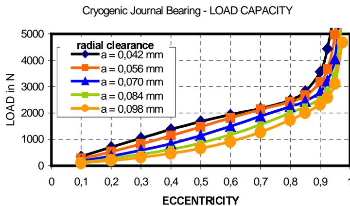
Figure 5: Influence of the radial clearance on the load
