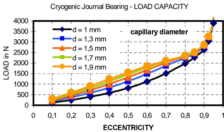
Figure 7: Influence of the capillary diameter on the load
