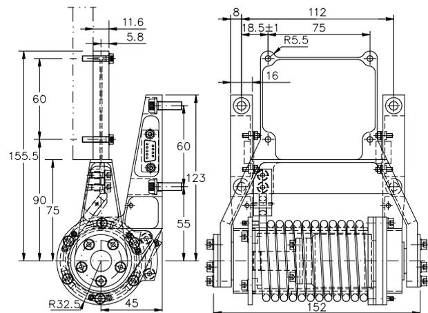
**Figure 7 Passive Hinge in Stowed Configuration**
