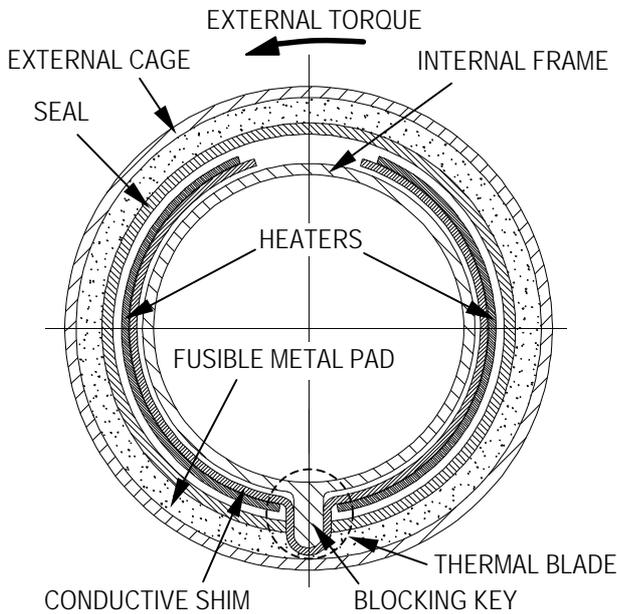
The deployment regulator concept consists of the following main parts:
