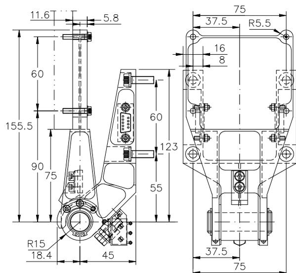
**Figure 8 Deployment Mechanism Deployed.**
