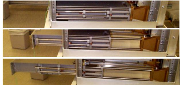
Figure 4. CWB Extraction Sequence
