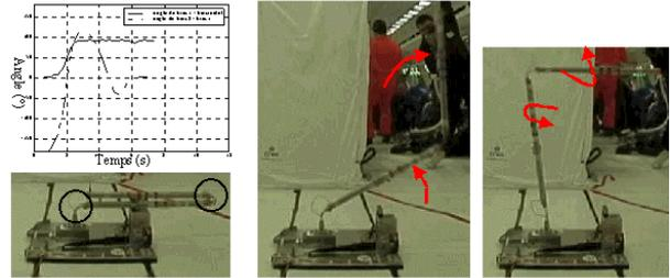
**figure 11: Micro-gravity two hinges / two arms deployment**
