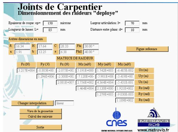
figure 2: Example of stiffness estimation issue from the model interpolation (simplified model in MATLAB<sup>®</sup> environment)
