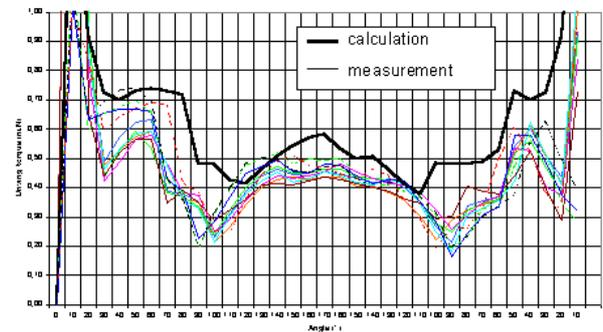
figure 8: Comparison between measured and calculated torques
