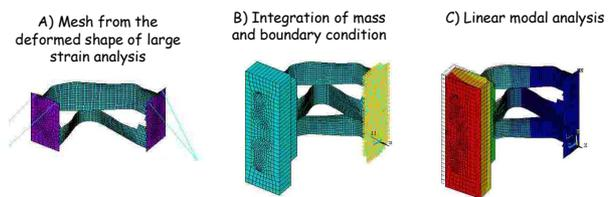
**figure 6: Procedure to estimate stiffness during opening**
