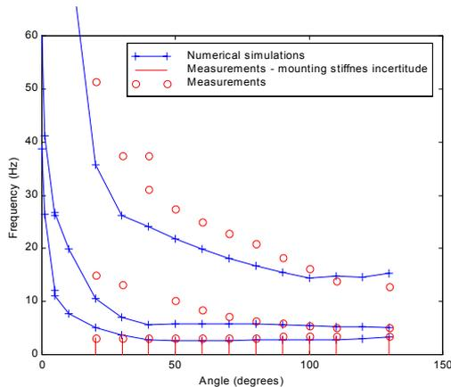
**figure 9: Comparison between measured and calculated stiffness\* vs opening angle (\* here, resonance frequencies in conditions described in figure 6)**
