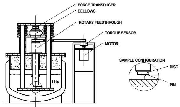
Figure 1. Cryotribometer CT 2
