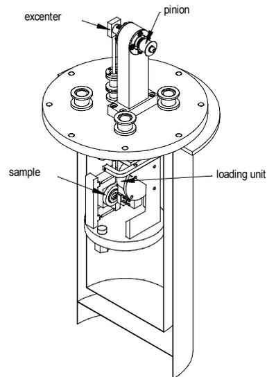
Figure 4: Cryotribometer for oscillating friction CT 4
