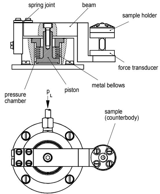
Figure 3: Combined loading and force measuring unit for low temperatures
