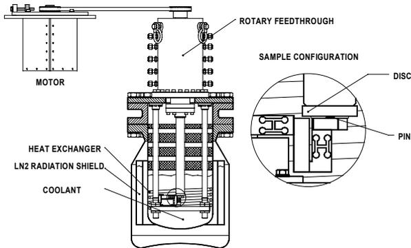
Figure 2: Cryotribometer and bearing test rig CT 3
