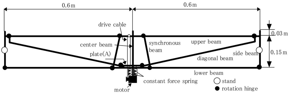
Fig.3 Planar truss
