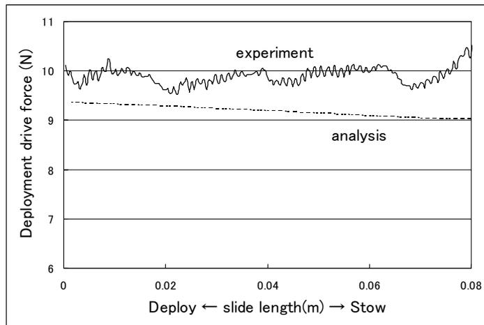
Fig.7 Estimation error due to analysis model
