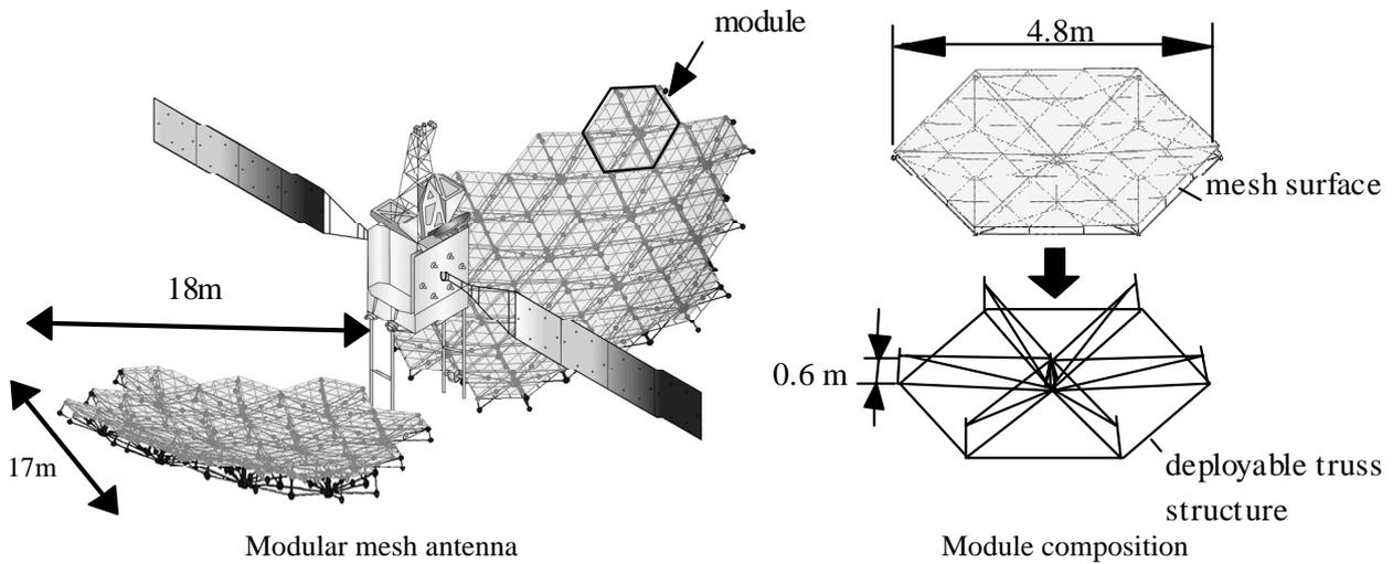
Fig.2 Modular mesh antenna
