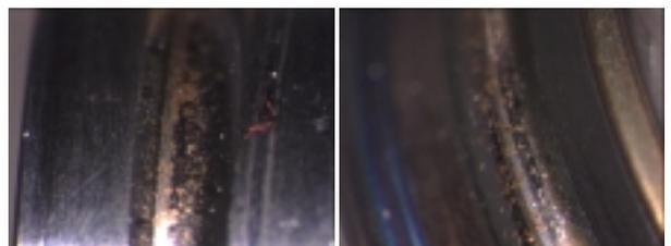
Figure 10 – bearing inner and outer race
