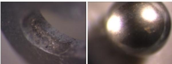
Figure 12 – bearing cage and ball
