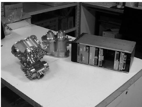
*Two ERV prototypes with controller*
