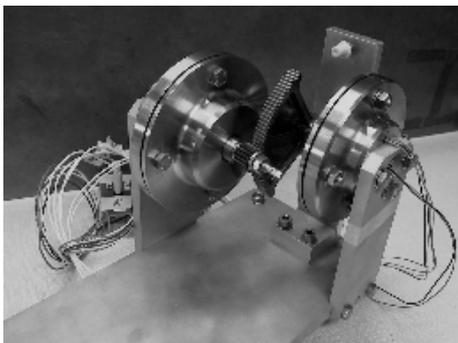
*Test tooling for debug of electronic driver*
