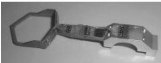
Figure 7: POD arm with bonded gauges
