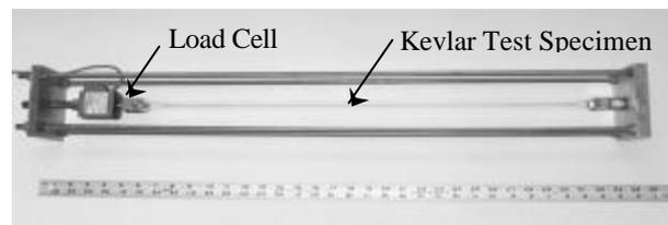
Figure 11: Test Specimen Load Relaxation Test Fixture
