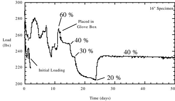
Figure 12: Load Over Time With Varying Relative Humidity
