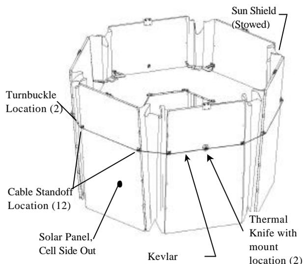
Figure 2: Stowed Configuration (Instrument not shown)
