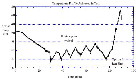
Figure 14: SARRS Cable Temperature Profile
