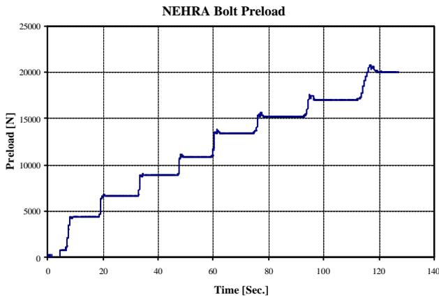
Figure 7. Bolt Preload up to 20 000 N
