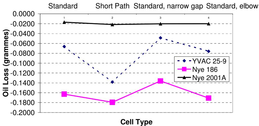
Table 4: Comparison of Measured Fluid Losses with Predictions
