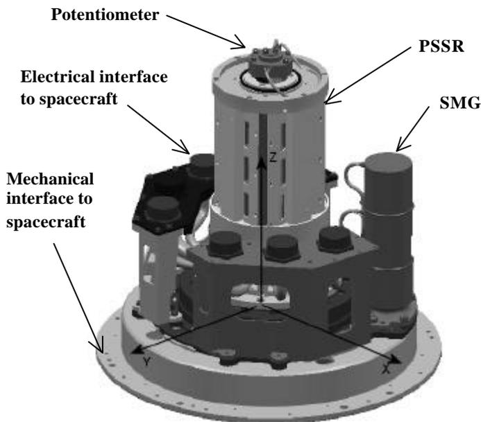
Figure 1: E3000 SADM showing the arrangement of the piece parts on the spacecraft side.
