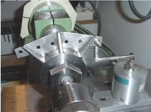
Figure 10, Roller screw friction torque measurement
