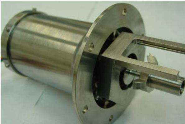
Figure 6, Stepper motor showing the piston of the decoupling system
