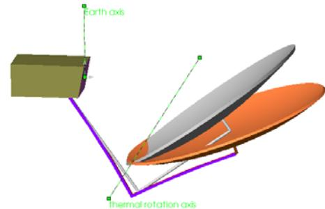
Figure 4: Assumed thermal distortion
