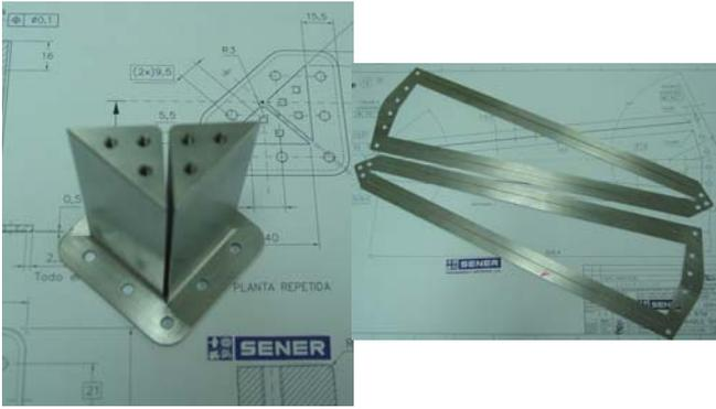
Figure 8, Torsion support structure and deformable INVAR sheets.
