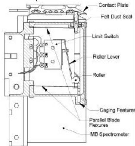
Figure 5. MB Contact Sensor
