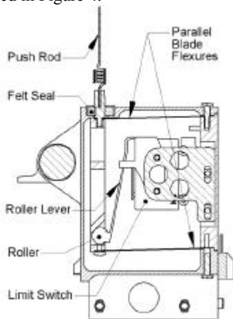
Figure 4. MI Contact Sensor
