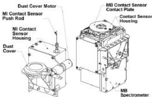
Figure 3. Contact Sensors and Dust Cover
