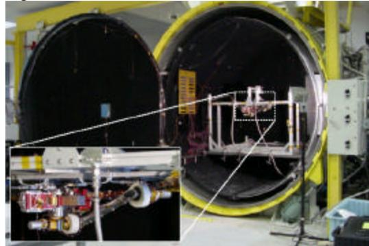
Figure 14. Thermal vacuum testing
