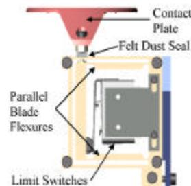
Figure 10. MB Contact Sensor
