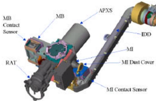
Figure 2. IDD with associated instruments
