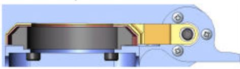
Figure 11. New Dust Cover Design (closed)
