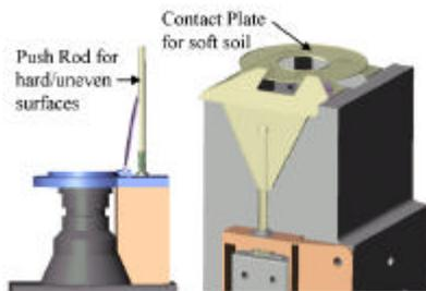
Figure 8. Designs optimized for rock & soil
