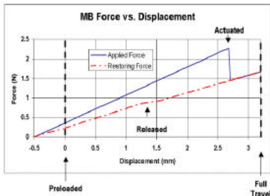
Figure 12. Contact sensor force vs. displacement
