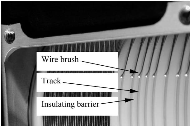
Figure VI. Close view of the wire brushes and slipping rotor of a medium power SRA.
