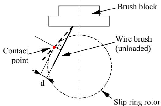
Figure VIII. Deflection  $d$  of a wire brush (working position) with respect to the unloaded position (adjusted position).
