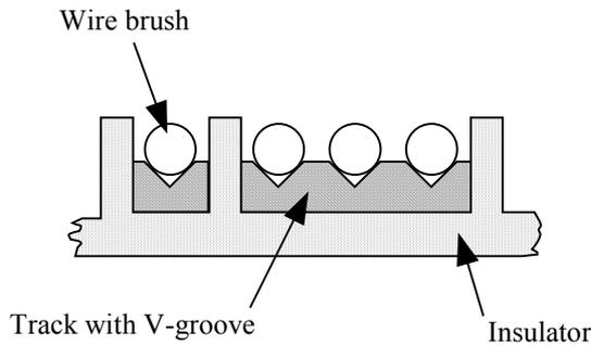
Figure V. Cross section of tracks and wire brushes. An example of three tracks at same electrical potential is presented.
