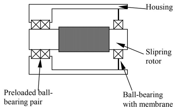
Figure III. Medium to high power SRA with conventional bearing arrangement.
