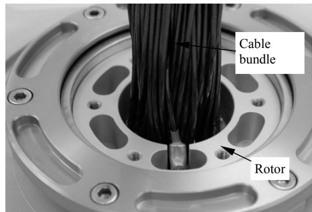
Figure VII. View of the cable loom output from the rotor of a SRA.
