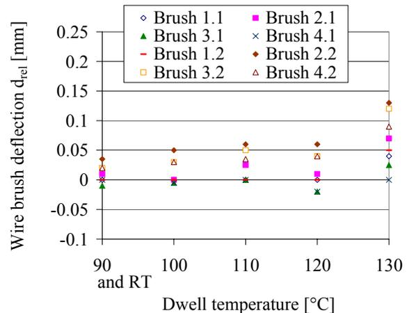
Figure XI. Variation of the wire brush unloaded deflection after different temperature dwells. The wire brushes are loaded at 50 mN during the thermal cycles. The relative deflection  $d_{rel}$  is given with respect to the nominal adjusted deflection  $d = 0.31 \pm 0.03$  mm in the present example.
