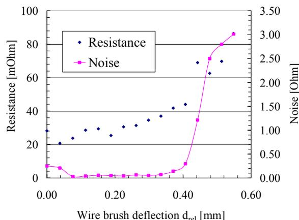
Figure IX. Effect of the wire brush preload on the contact resistance and on the electrical noise. The relative deflection  $d_{rel}$  is given with respect to the nominal adjusted deflection  $d = 0.5 \pm 0.05$  mm in the present test. The noise is a peak to peak value.
