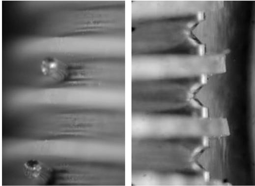
Figure XII. Close view of tracks and wire brushes after an accelerated lifetime test under vacuum (4.5 A per track, 10'000 revolutions).
