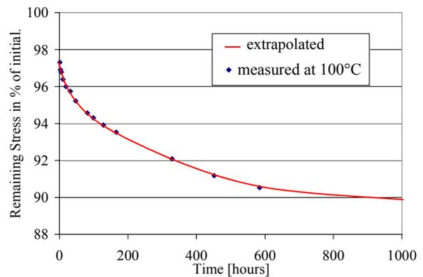
Figure XIII. Decrease of the adjusted elastic stress in the used gold alloy as a function of time.
