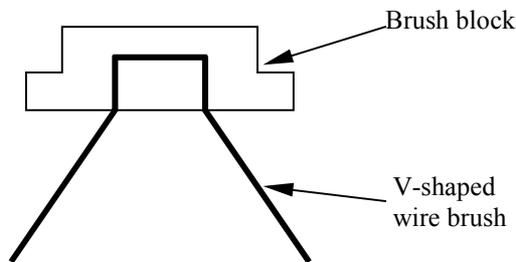
Figure X. Scheme of the geometry of a V-shaped wire brush.
