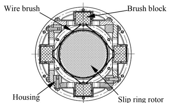
Figure IV. Section of a typical medium to high power SRA. Four brush blocks with each double V-shaped wire brushes per track are present on this design.
