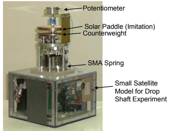
Fig. 2 Solar paddle actuator fixed on small satellite model.
