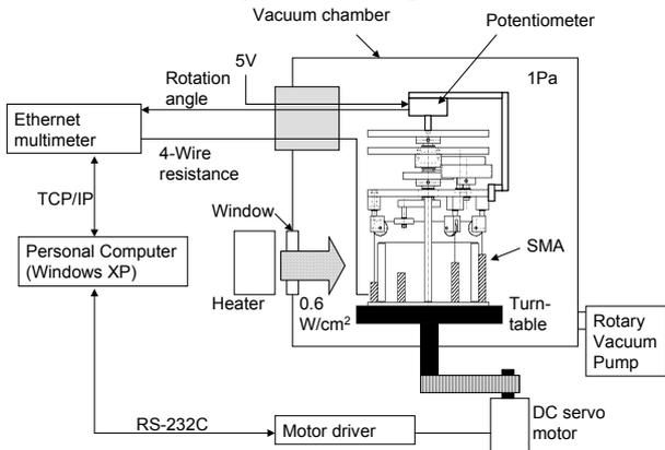
Fig. 5 Block diagram of vacuum experiments.
