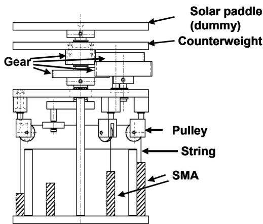
Fig.1 Solar paddle actuator.
