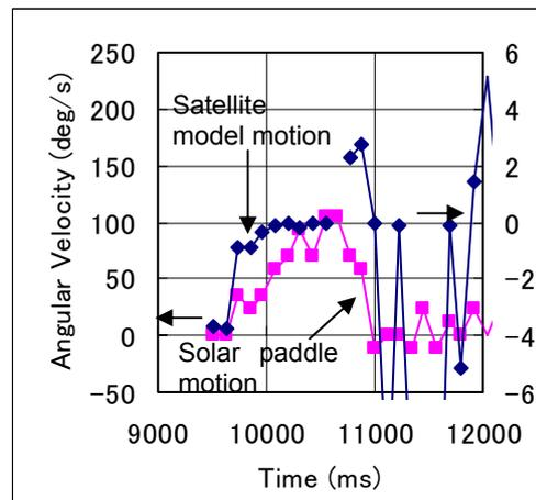
Fig. 4 Motion results without counterweight.
