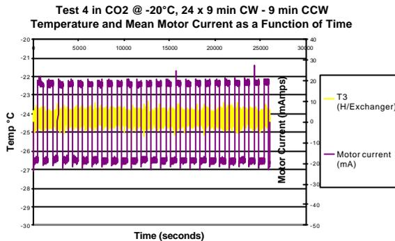
Figure 6: Example of motor current for life test
