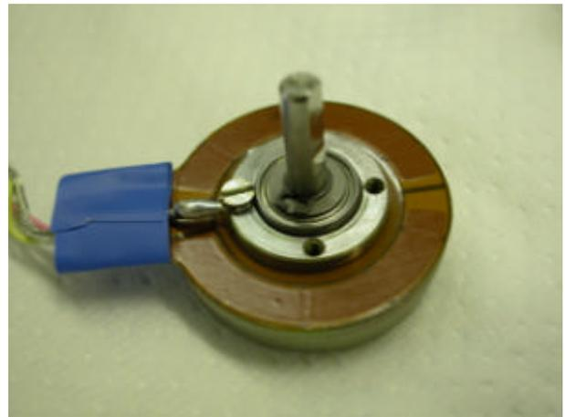
Figure 8: Shinsei Rotary Piezomotor
