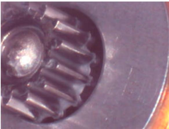
Figure 7: Maxon motor pinion following life-test
