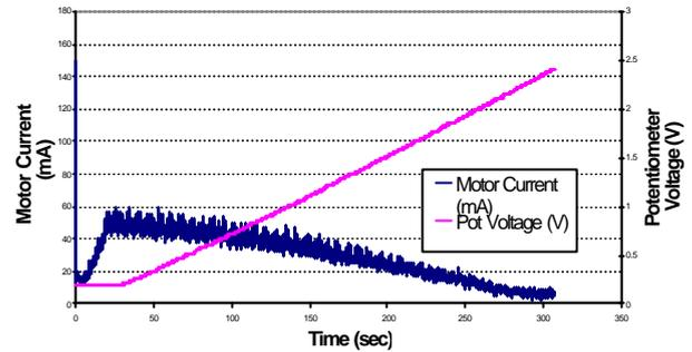
Figure 5: Example of Main Hinge deployment motor current as it lifts simulated base load from horizontal to 95 deg
